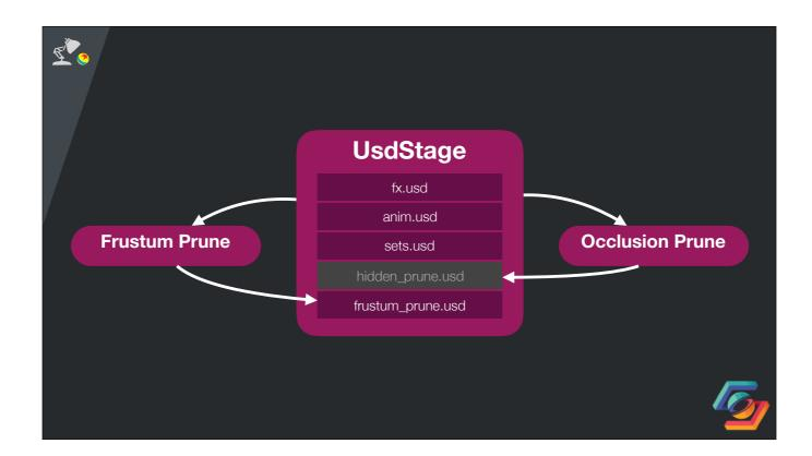
Using libwork and Intel's TBB are great for CPU parallelism for our frustum prune. But for our occlusion prune, we'd really like to advantage of GPU Parallelism via Hydra's Storm renderer.
